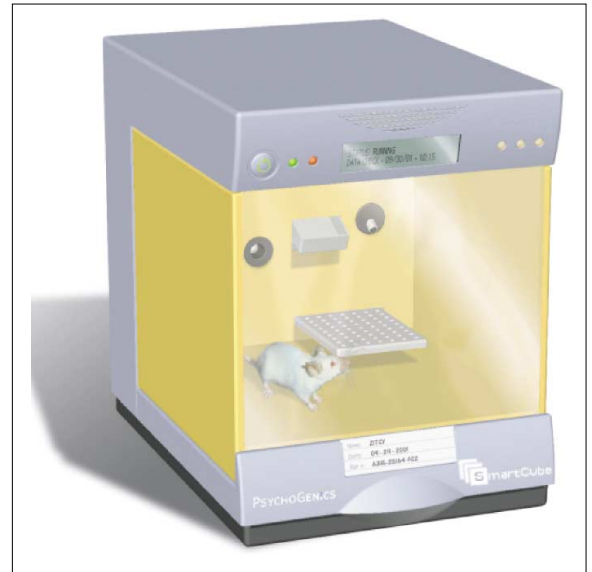
Fig. 1. The SmartCube™ system (PsychoGenics, Inc., patent pending) will be the first to automatically and systematically capture, quantify and store information on a large number of behavioral motor and posture patterns exhibited by genetically altered or pharmacologically manipulated mice in a high-throughput manner. The SmartCube™ will incorporate robot-like hardware, computer vision, neurological assessment tools and machine-learning algorithms to capture and integrate behavioral and physiological parameters. In addition to the usual measures of frequency, duration and intensity of numerous behaviors, the system will also analyze complex patterns such as transition matrices (i.e. the temporal succession of different behaviors). Physiological parameters, such as heart rate, can also be quantified, in parallel with the acquisition of behavioral data. (With permission from PsychoGenics Inc.)
